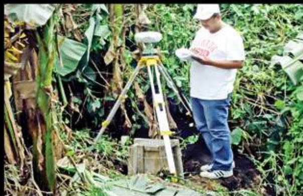
Cadastral surveys are conducted to determine the "metes and bounds" of all parcels within an entire municipality or city for land registration and other purposes
