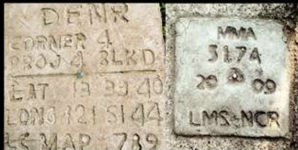
A control point is an accurately surveyed coordinate location for a physical feature that can be identified on the ground.
