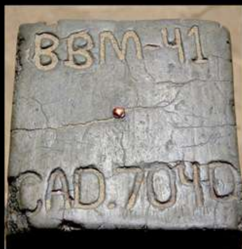
Sample of a reference marker where the point of beginning of the polygon of the land parcel is connected. The position of the lot is fixed in relation to this monument using bearing and distance. It is commonly called as the "tie point" of the lot.
